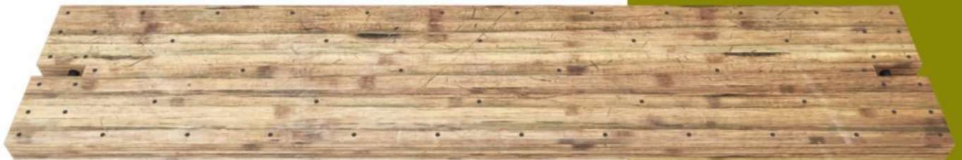
HORIZONTAL LAMINATED BAMBOO LAYERS
